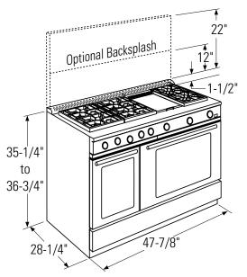
Clearances between range and side wall or combustible material must be at least 12" on each side.
